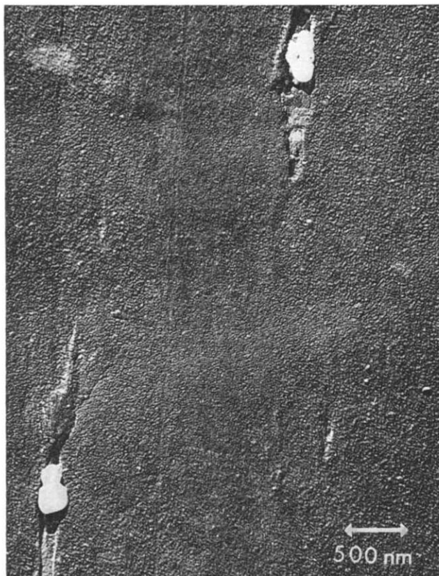
Figure 2 Chromium replica of a polyester filament surface showing exposed titanium pigment (S.C.S.)
