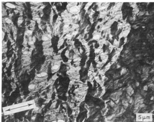
Figure 12 Transmission electron micrograph of a strained microtomed section of compression moulded TPX. The arrows indicate the stretching direction
