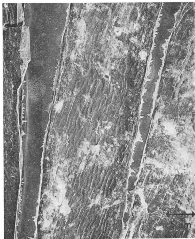
Figure 4 Carbon replica (Chippendale technique) illustrating the removal of a deposit from cotton fibres (S.C.S.)
