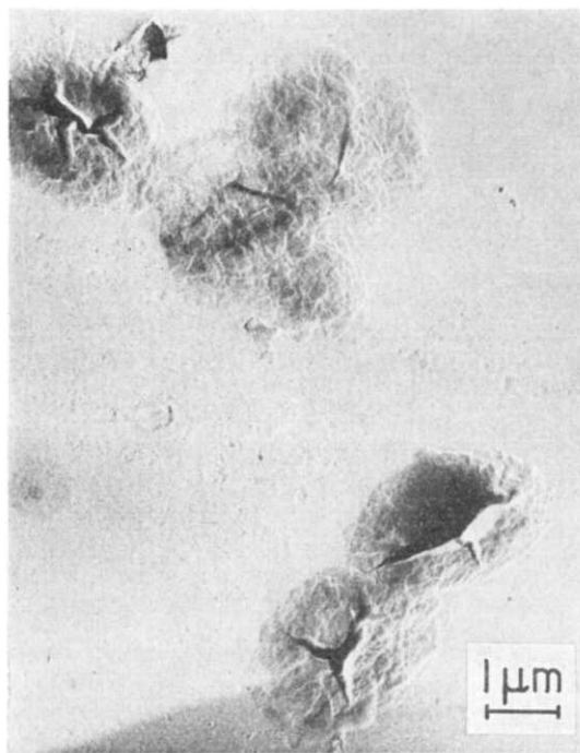
Figure 6 Seeded single crystals of PCO-3 from DMF; c=2.0 \times 10^{-2}\% ; T_{sol}=99^{\circ}\text{C} ; T_{cc}=21^{\circ}\text{C} ; T_s=84.5^{\circ}\text{C} ; T_c=42^{\circ}\text{C}
